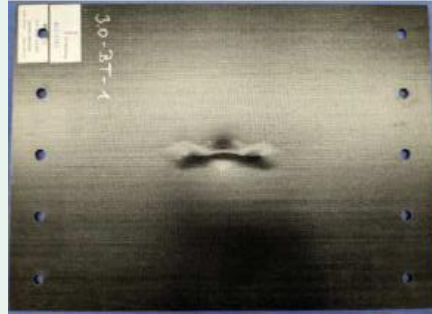
3.0 Sandwich with PP-GF30 core
