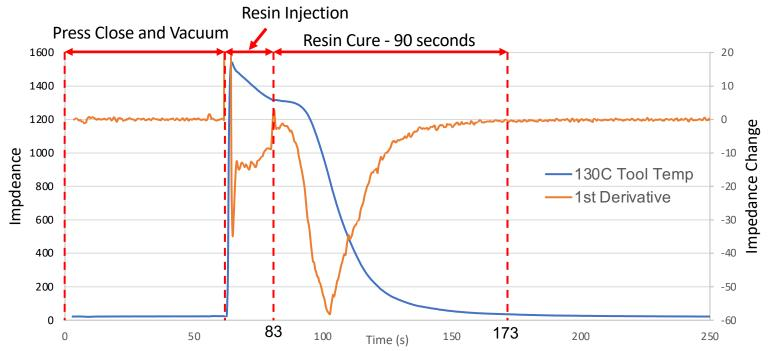
Demolding at between a 200-250s cycle time should be feasible (120-150s resin cure time) Minimal change in material impedance or rate of change during this time frame
