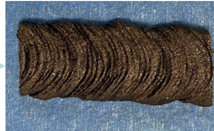
13 wt % Carbon fiber reinforced ABS 3D printed using LAAM system
