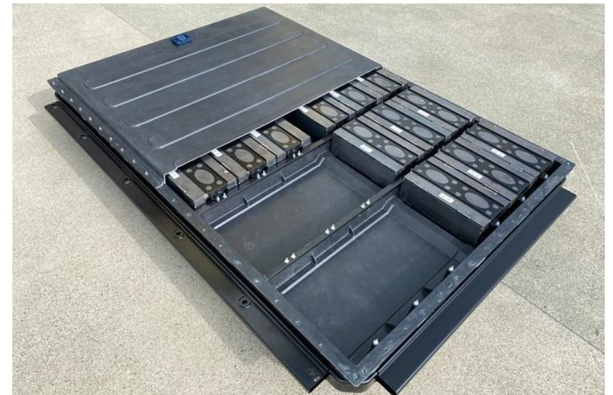
Battery enclosure panel
