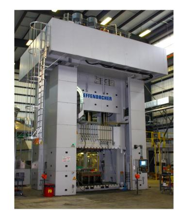
□ SMC Line and 2500 tonne hydraulic press
