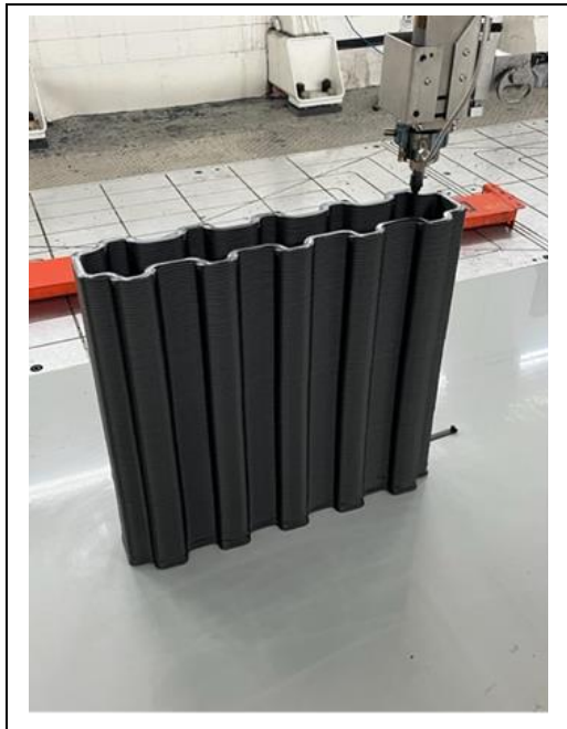
Figure 2: Top hat sections being printed in vertical orientation
