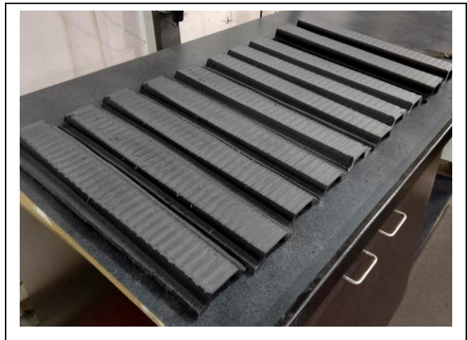
Figure 3: Top hat sections after separation and surface finishing
