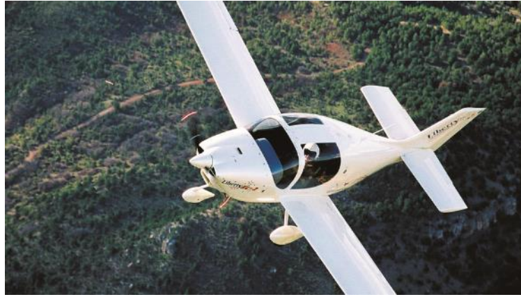
Fuselage PEI foam Carbon pre-preg, autoclave
