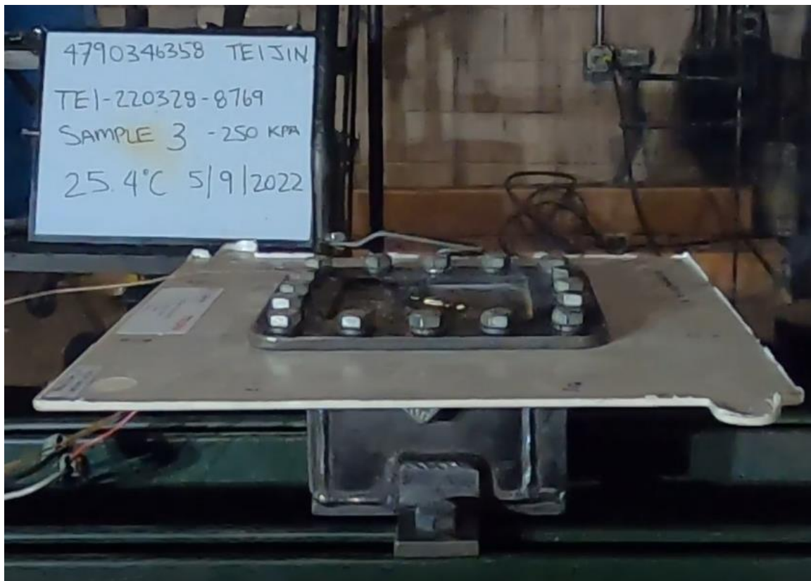
Figure 6. Intumescent SMC sample after UL 2596 testing
