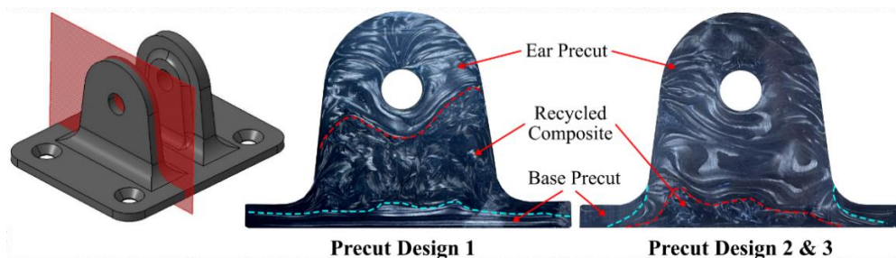
Figure 8: The microscopic image of cross-sectional area of the pin brackets fabricated with the precut design 1 and 2 & 3.
