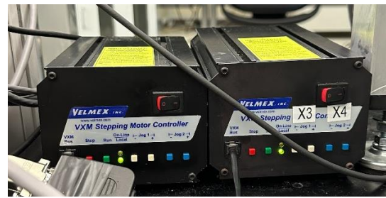
Figure 3: Velmex system to control the movement of transducer
