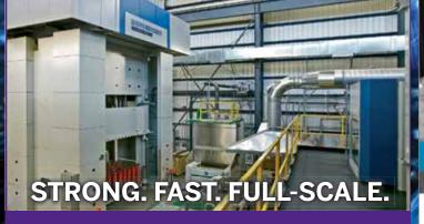
At the **Fraunhofer Innovation Platform for Composites Research at Western**, our 2,500t industrial hydraulic press develops technologies that incorporate the strength of aerospace composites and the fast cycle time of automotive components.
