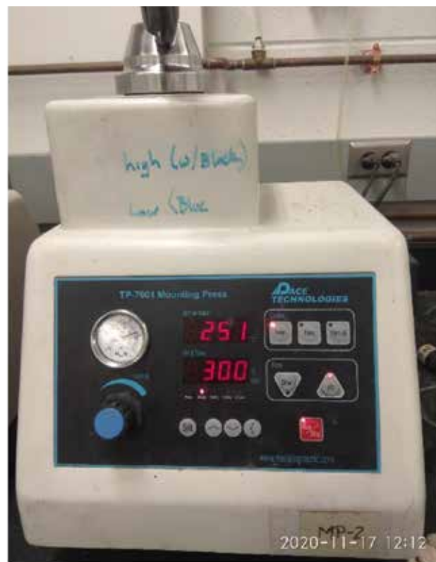
Figure 1. Heat compression mounting equipment used for fabrication of composites.
