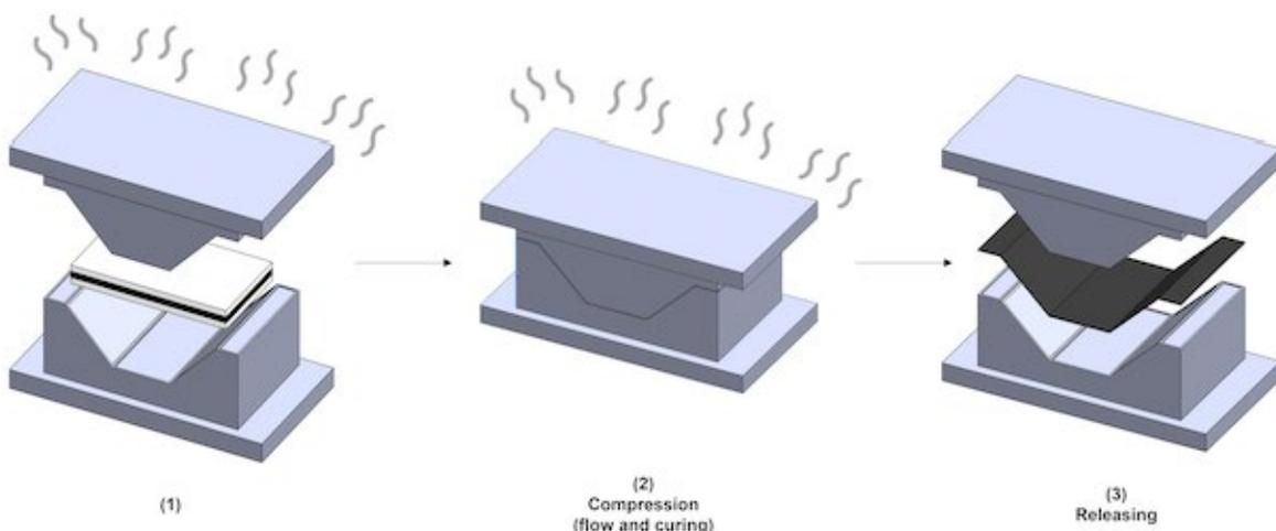
Figure 1: The sheet molding compression process. Adapted [14].
