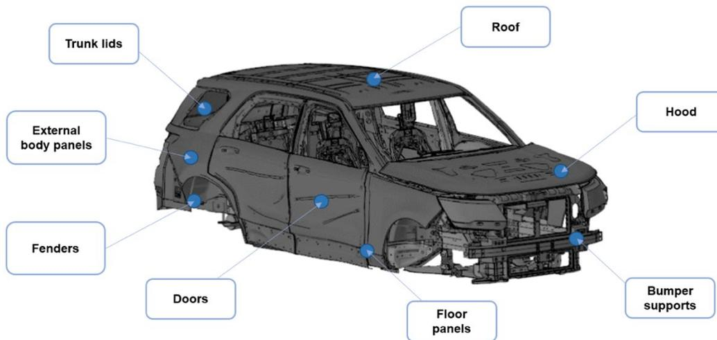
Figure 2: SMC Structural parts.
