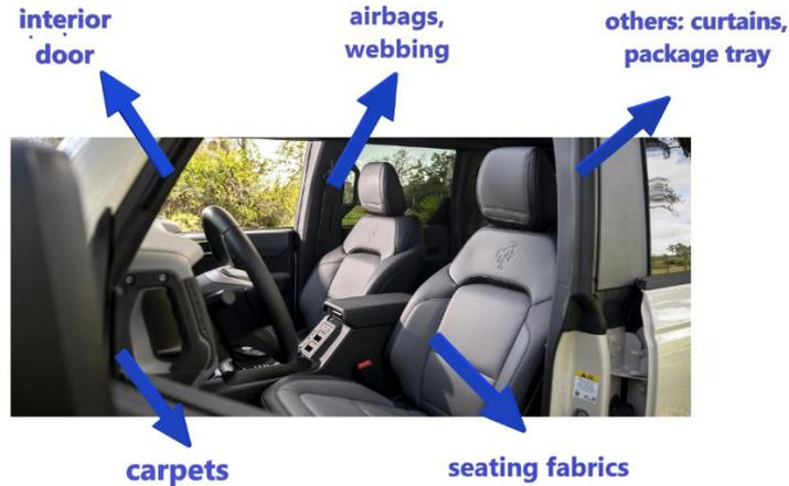
Figure 1: Some potential applications for textile composites in interior car body.
