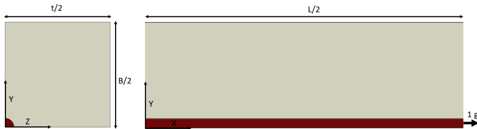
Figure 7. FE model for single fiber fragmentation ( t/d \approx 14.5 , L/d \approx 285 ).
