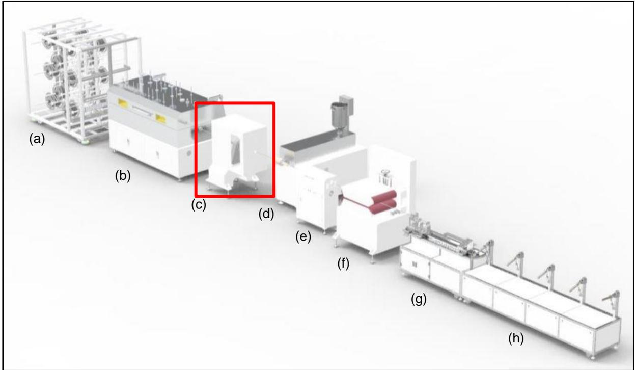
Figure 1: Overview of M-TOW<sup>®</sup> line. Components shown include a) creel, b) oven, c) braider, d) extruder, e) cooler, f) puller, g) cutter, h) stacker. Image courtesy of EELCEE Ltd [13].
