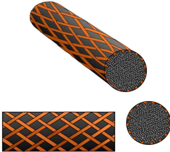
Figure 2: Representation of M-TOW® with 16 wires of copper overbraided. The glass fibers in the prepreg consolidate to the center of the tow while the wires embed into the surface polymer to create a circular rod/tow.
