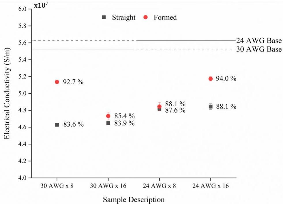
Figure 6. Electrical conductivity of functional M-TOW<sup>®</sup> compared before (straight) and after (formed) forming. Fractional conductivities with respect to the baseline value are labelled. Error bars represent one standard error of the measurement set.
