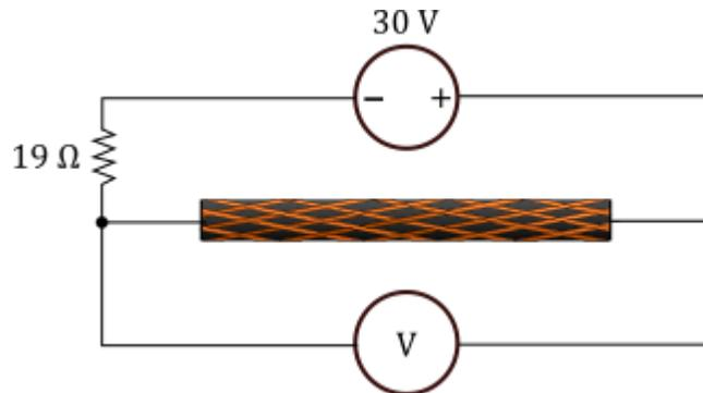
Figure 4. Schematic of test setup for the determination of the M-TOW® electrical conductivity. A constant 30 V DC power supply was used while a voltmeter measured the voltage drop across the sample.
