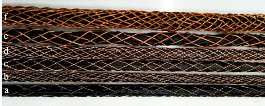
Figure 3: M-TOW® samples with overbraided copper wire. From bottom to top: a) 30 AWG x 8, b) 30 AWG x 16, c) 24 AWG x 8, d) 24 AWG x 16, e) 18 AWG x 8, f) 18 AWG x 16.
