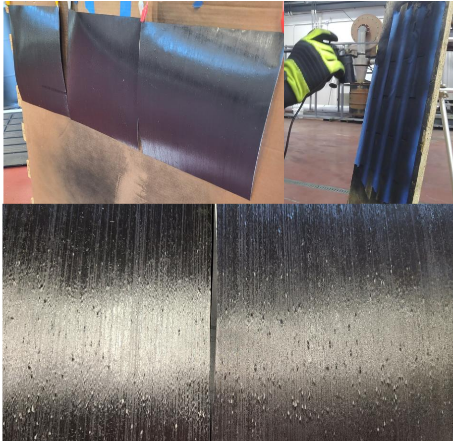
Figure 4: Spray coating of CF/epoxy prepreg sheets.
