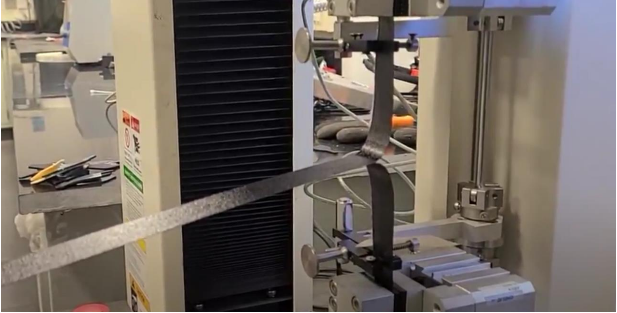
Figure 8: T-Peel testing of pGNP/CF/epoxy composites.
