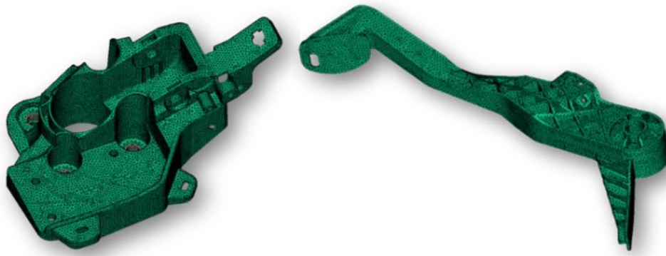
Figure 2- Pedal box and Brake pedal
