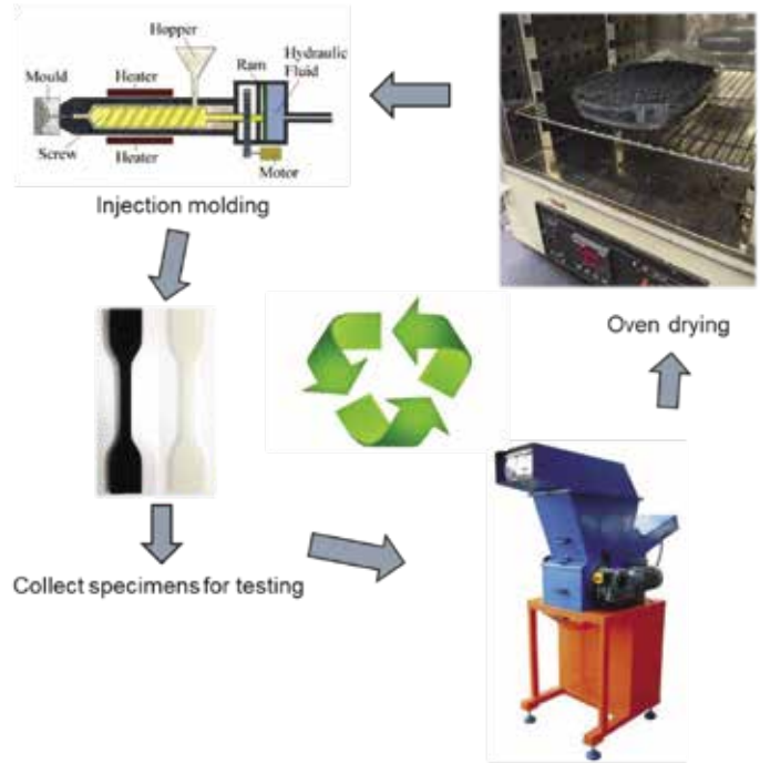
Figure 1 Recycling steps used in this study for thermoplastic composites
