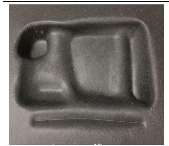
Figure 5: Scrim A molded in wrinkle tool
