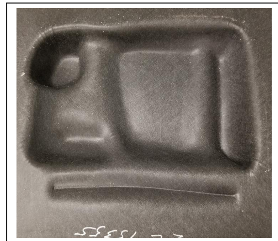
Figure 7: Scrim C molded in wrinkle tool
