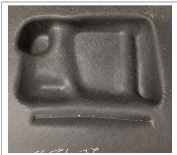
Figure 6: Scrim B molded in wrinkle tool
