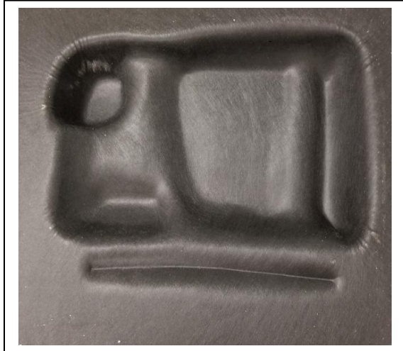
Figure 4: Existing Scrim molded in wrinkle tool
