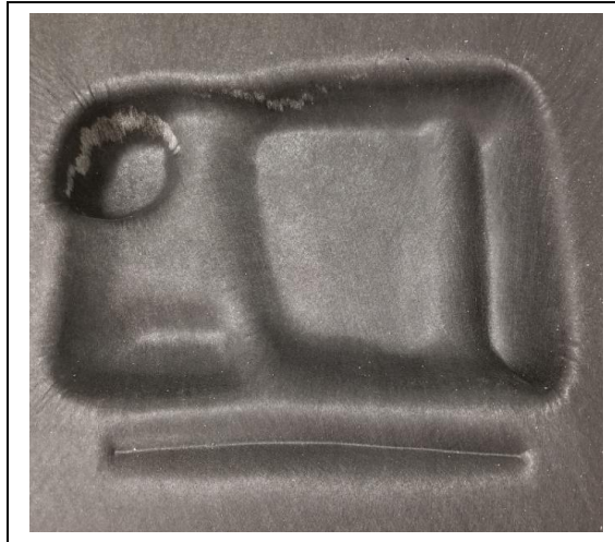
Figure 8: Scrim D molded in wrinkle tool
