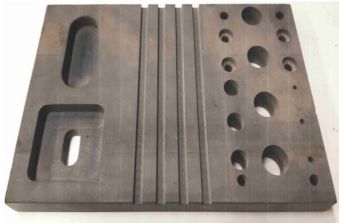
Image 7. Composite panel after all machining
