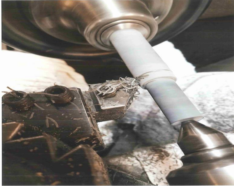
Image 8. Turning a block of composite
