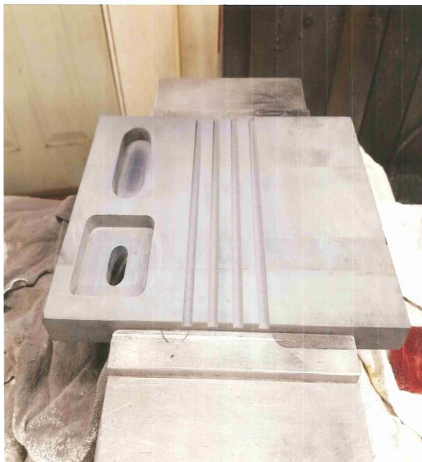
Image 5. Composite panel after all milling
