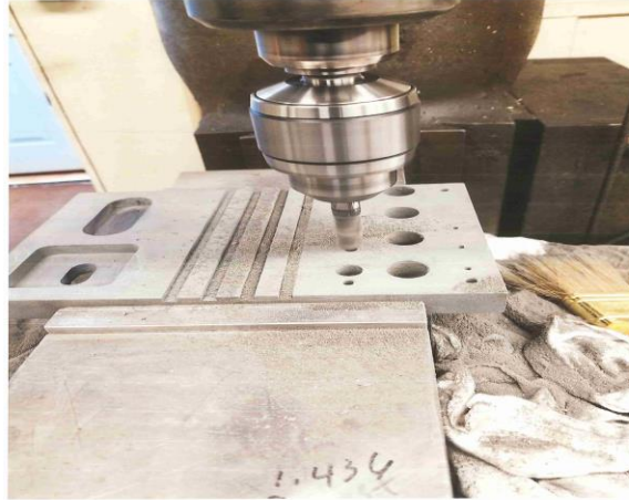
Image 6. Drilling of epoxy composite panel
