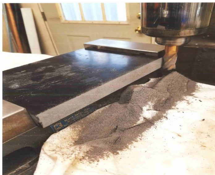
Image 3. Side milling of composite panel
