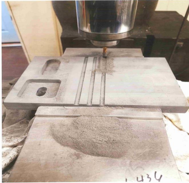
Image 4. Routing in the composite panel
