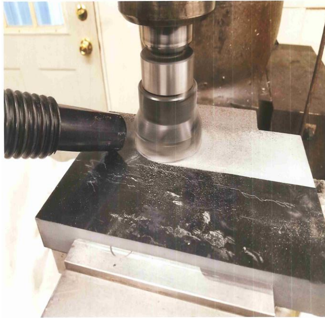
Image 2. Surface milling of composite panel
