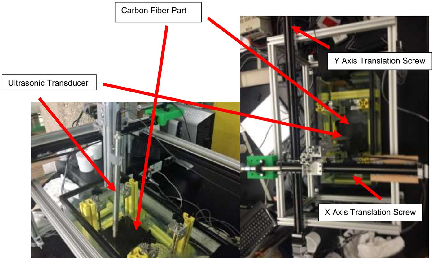
Figure 3: Custom ultrasonic Set-up.
