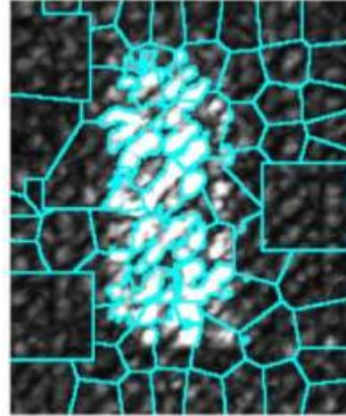
Figure 8: Superpixels superimposed over C-scan Image
