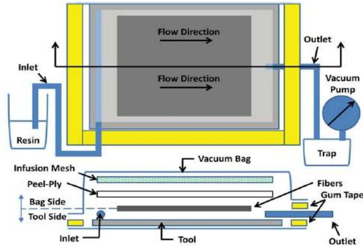
Figure 1: Diagram of VARTM process
