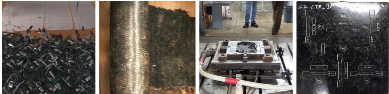
Figure 2 Epoxy / Carbon SMC fabrication process: a) sheet compounding b) roll maturation c) compression molding d) panel testing
