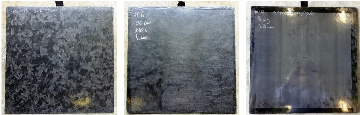
Figure 3 Sample SMC panels a) baseline b) spread tow c) co-cure sandwich
