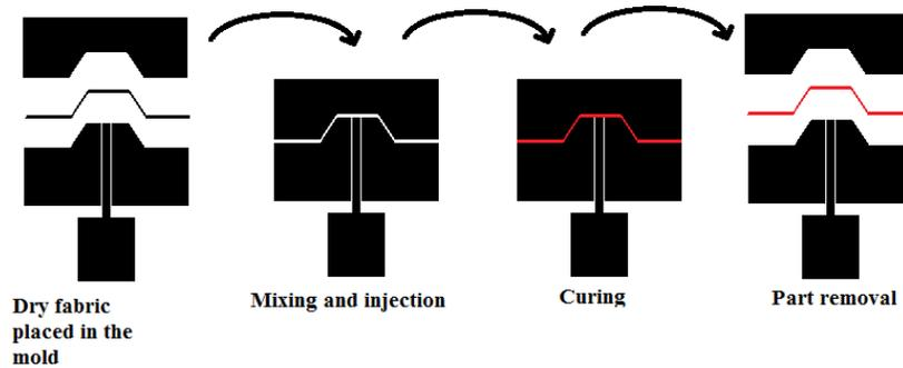
Figure 1 – Schematic representation of HP-iRTM process.
