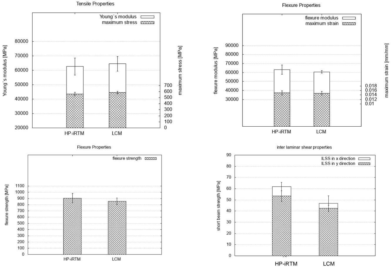
Figure 7– Tensile, Flexure and ILSS mechanical tests results
