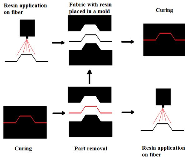
Figure 2 – Schematic representation of LCM process.
