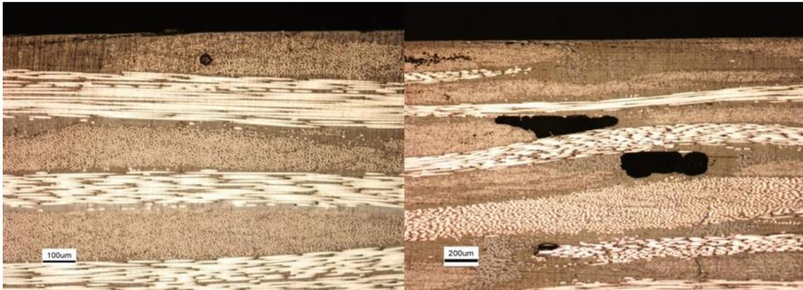
Figure 6– Light microscopy results. HP-iRTM sample on the left and LCM sample on the right
