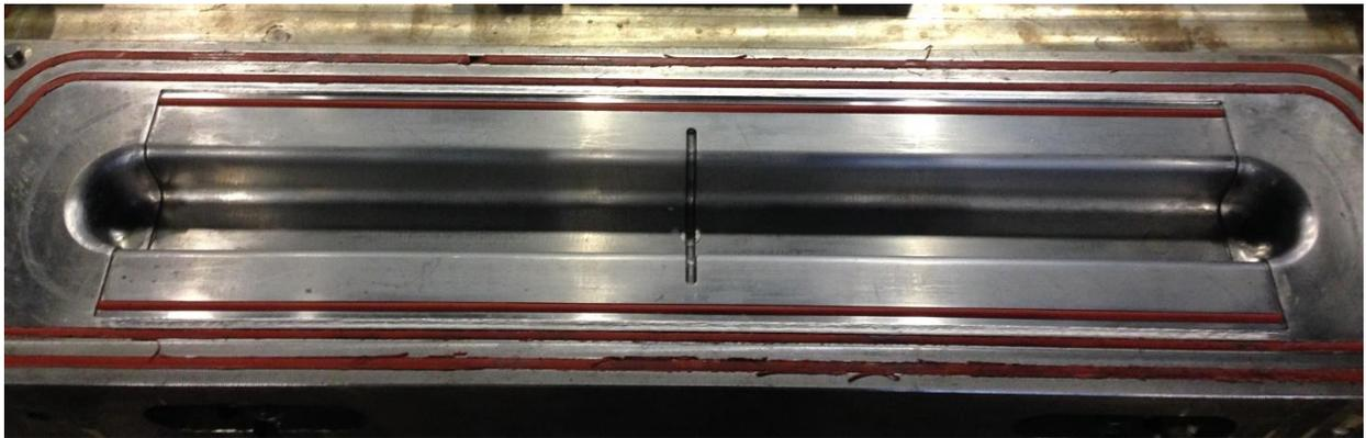
Figure 4 – HP-iRTM C-channel mold
