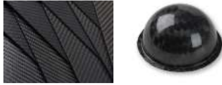
Figure 4: Lamination Sheets and a Formed Lamination Sheet from SPIC co.
