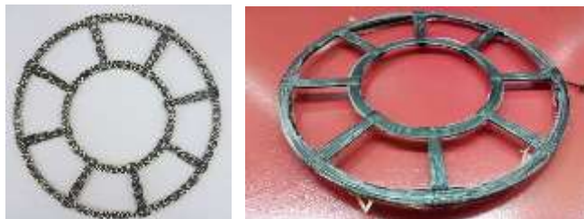
Figure 11: Simulated Propeller; Fiber Laying Prepreg (left) from Tajima Group, and Light Molding (right) from D-MEC Ltd.
