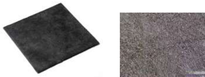
Figure 6: Non-Woven Cloth of Carbon Fiber and XD10 fiber (left). Enlarged View of the Cloth (right) from ITC co.
