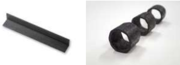
Figure 10: Pultrusion Molding Samples Made from UD Tape (left) and Commingled Yarn (right).
