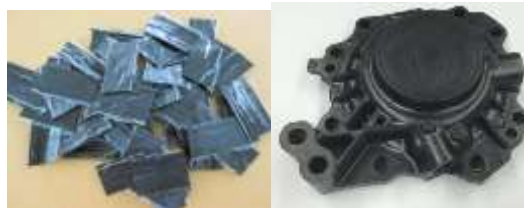
Figure 8: Chopped UD Tape (left) and Its Compression Molding of a Part of Motorbike (right) from Hamamatsu Society of CFRP Business R&D.
