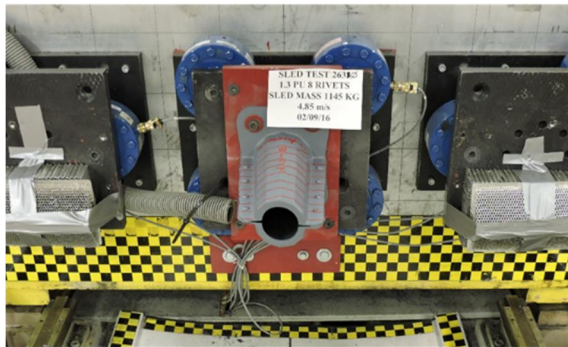
Figure 11: Image of a crush can ready to be impacted. Four load cells are used to track the force during the impact. The crush can is mounted stationary on the wall while the sled travels along rails to impact it. The impactor weighed 1145 kg and traveled at 4.85 m/s at the time of initial impact.
