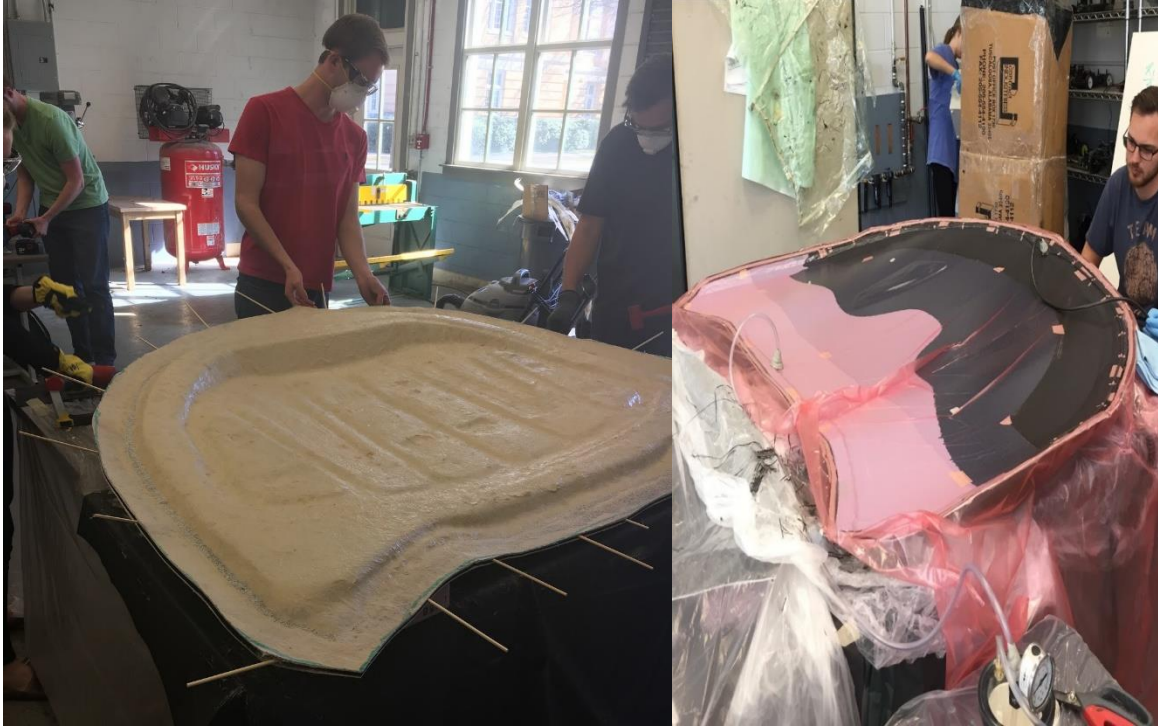
Figure 2: Picture of the mold (left) and of the vacuum forming process (right) used to make the prototype hood.
