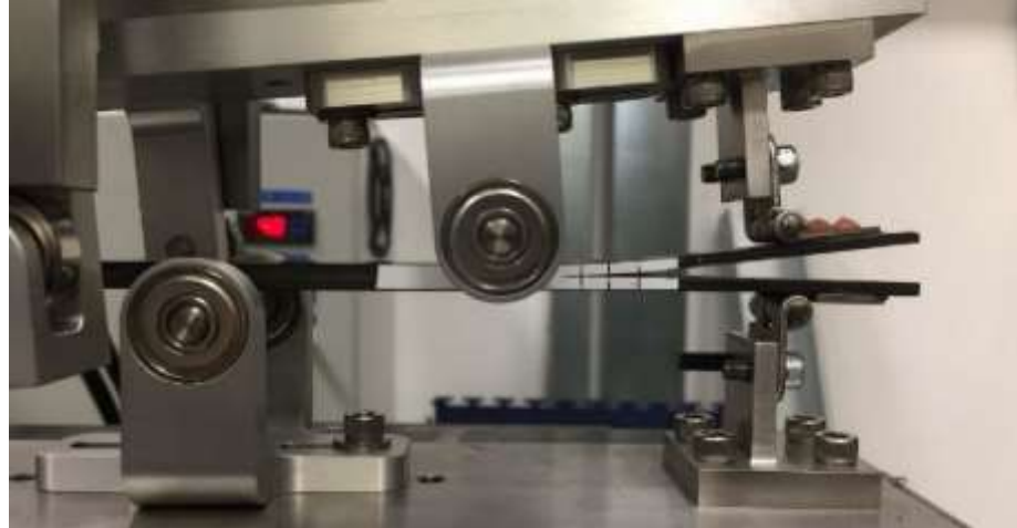
Figure 4: Test Setup for Mixed-Mode Bending
