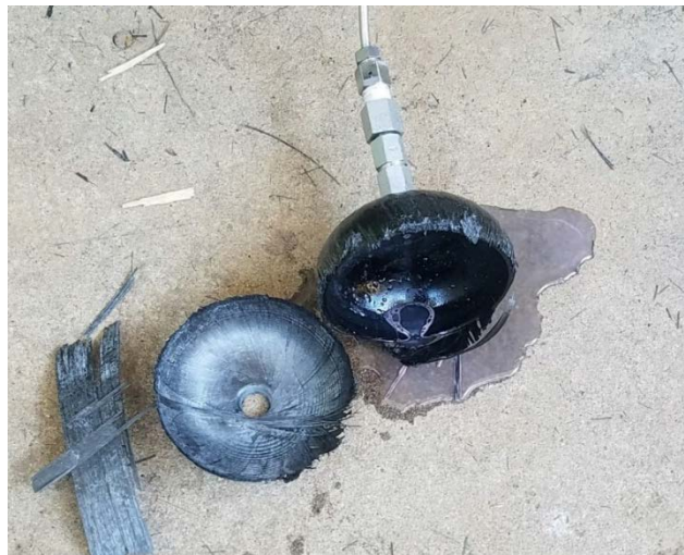
Figure 4: Burst Recycled pressure vessel (737 bar)
