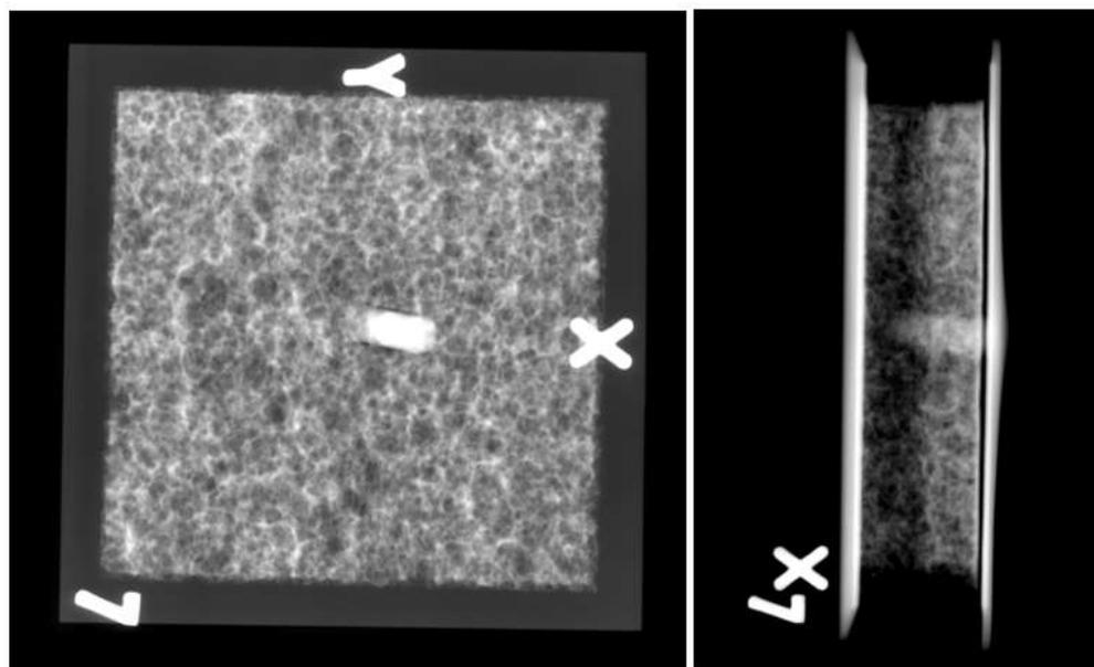
Figure 13: Post-impact radiography images of sample S-1.
