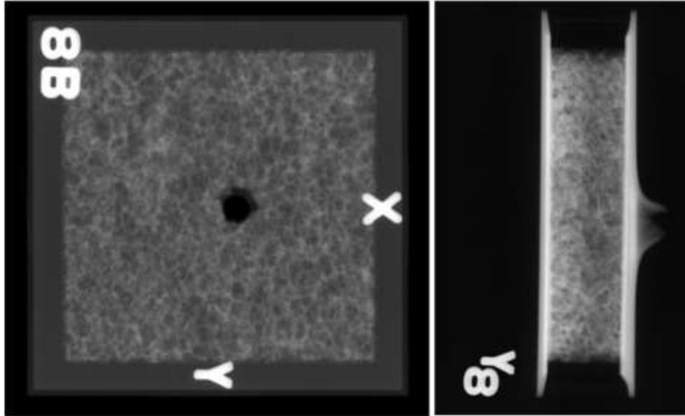
Figure 16: Post-impact radiography images of sample S-2.
