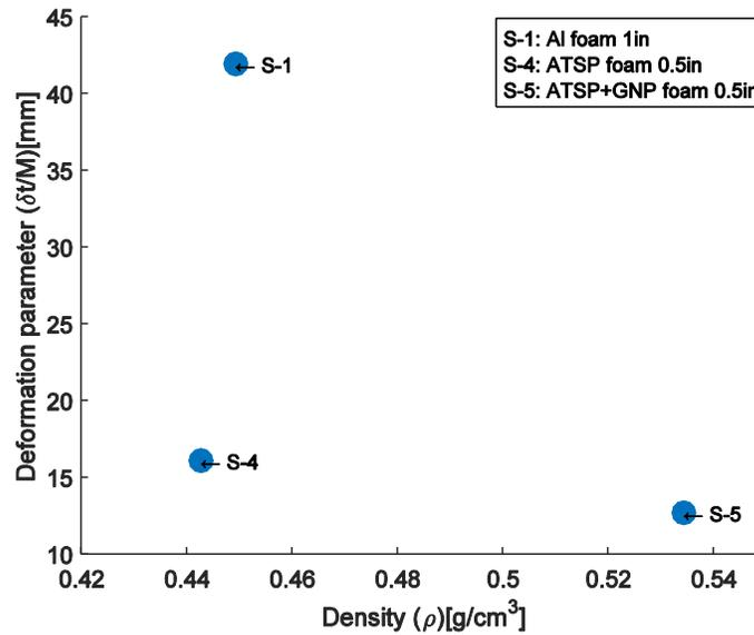
Figure 1: Quantification plot for samples S-1, S-4, and S-5 that exhibited penetration damage.
