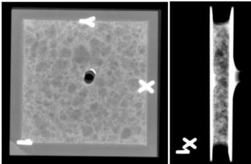
Figure 28: Post-impact radiography images of sample S-6.
