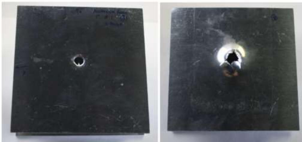
Figure 15: Post-impact top and bottom views of sample S-2.
