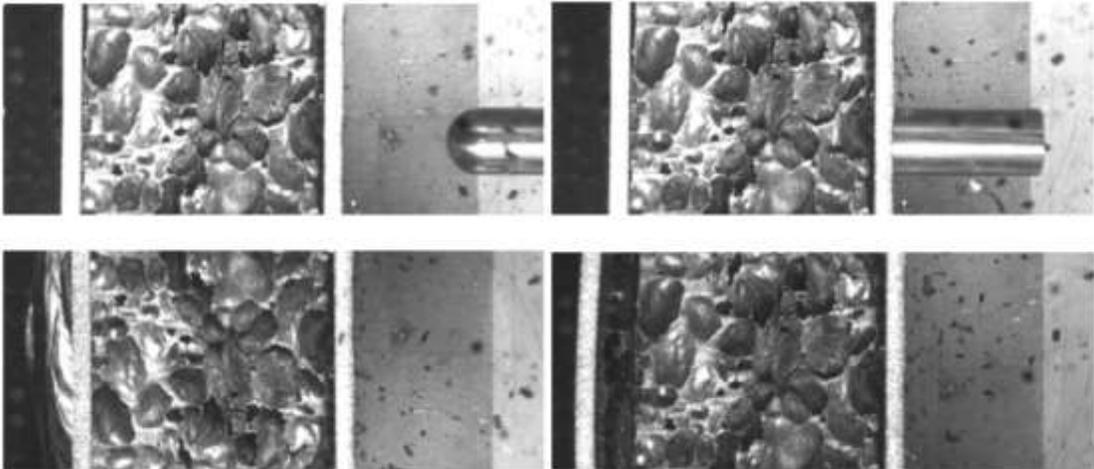
Figure 6: High-speed time lapse image of test case corresponding to sample S-1, ordered from top left to bottom right - 292.9m/s.
