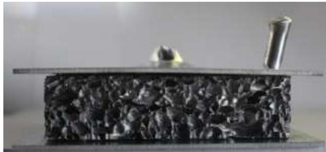
Figure 14: Post-impact side view image of sample S-2.
