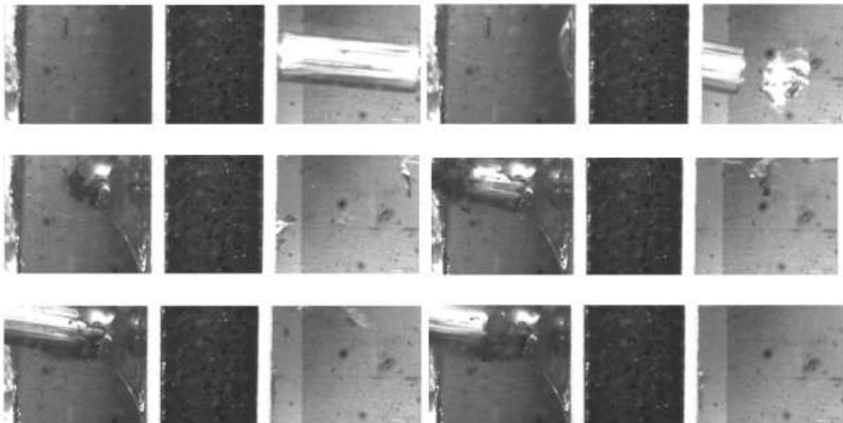
Figure 11: High-speed time lapse image of test case corresponding to sample S-6, ordered from top left to bottom right – 344.7 m/s.
