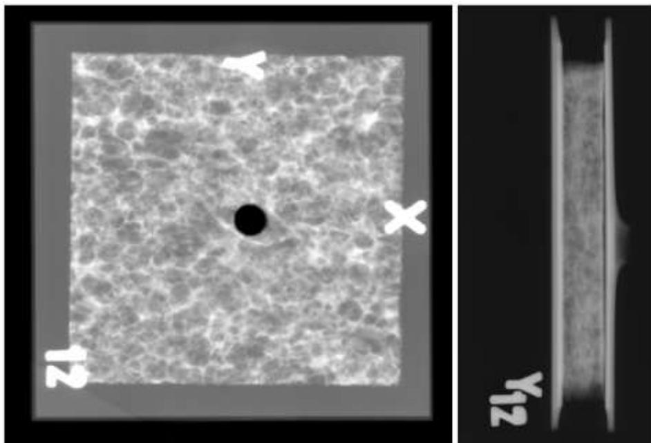
Figure 19: Post-impact radiography images of sample S-3.
