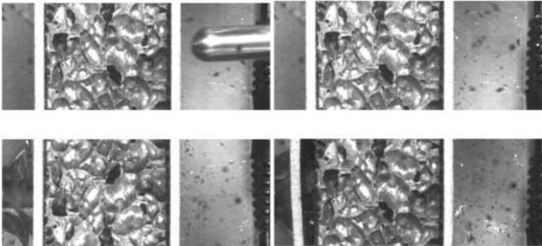
Figure 7: High-speed time lapse image of test case corresponding to sample S-2, ordered from top left to bottom right – 403.3m/s.
