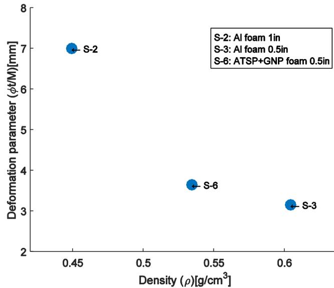
Figure 30: Quantification plot for samples S-2, S-3, and S-6 that exhibited perforation damage.
