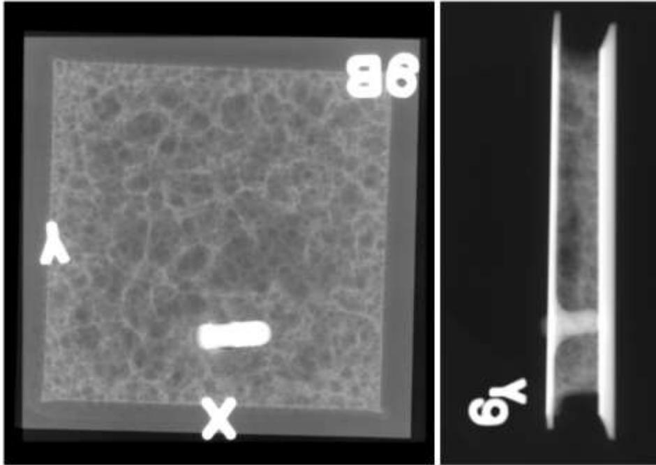
Figure 25: Post-impact radiography images of sample S-5.
