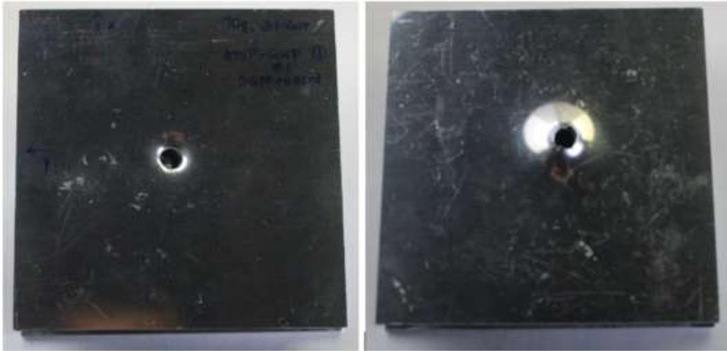
Figure 27: Post-impact top and bottom views of sample S-6.
