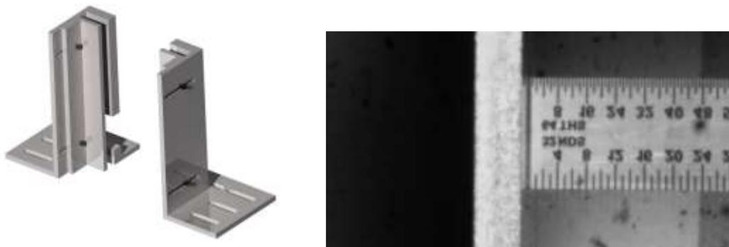
Figure 5: L-clamps used to hold the sample and a high speed image with a fiducial marker.
