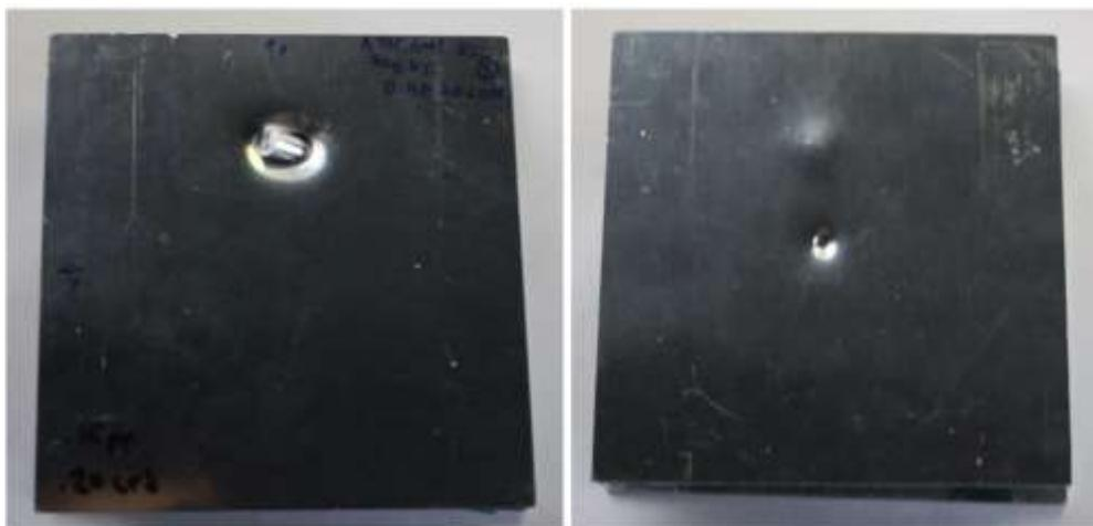
Figure 24: Post-impact top and bottom views of sample S-5.
