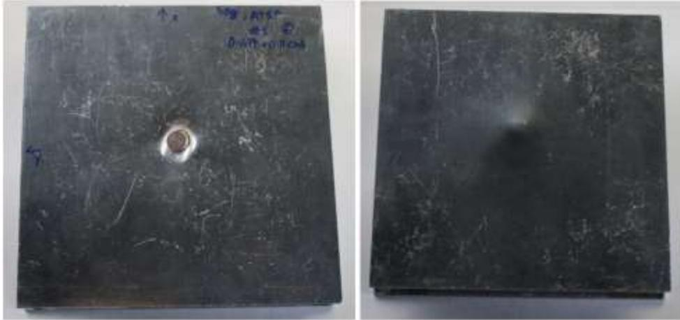
Figure 21: Post-impact top and bottom views of sample S-4.
