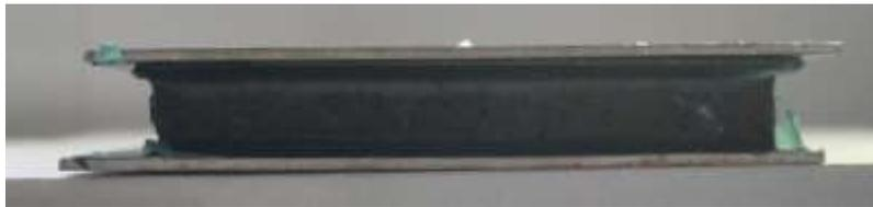
Figure 23: Post-impact side view of sample S-5.
