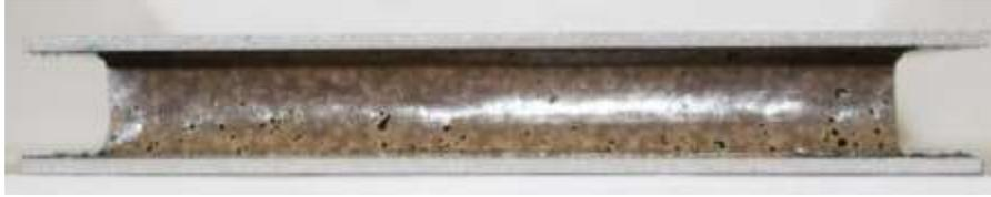
Figure 1: ATSP foam core sandwich panel.
