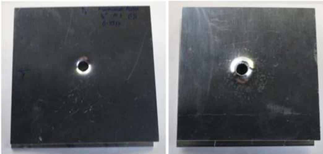
Figure 18: Post-impact top and bottom views of sample S-3.
