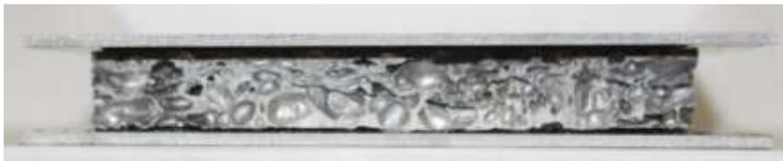
Figure 3: Half-inch thick aluminum foam core sandwich panel.
