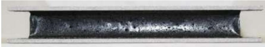
Figure 2: ATSP foam core sandwich panel infused with 3wt% GNP.
