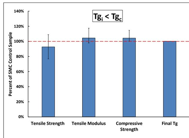
Figure 3: Relative properties comparison between SMC control material and molding compound prepared from the trim scarp when the trim scarp  $Tg_i < Tg_c$
