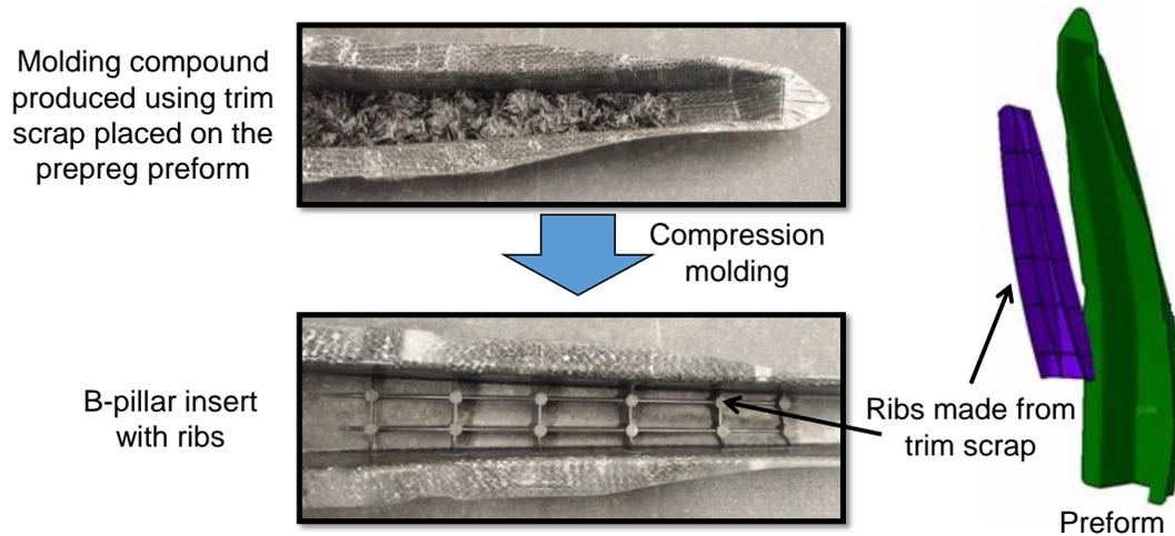
Figure 6: Illustration of co-molding the reclaimed prepreg scrap with virgin prepreg
