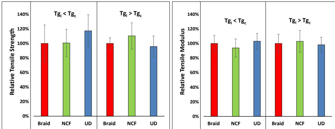
Figure 5: Relative tensile properties comparison (left) tensile strength, and (right) tensile modulus of parts made from trim scraps of three types of prepreg fabric
