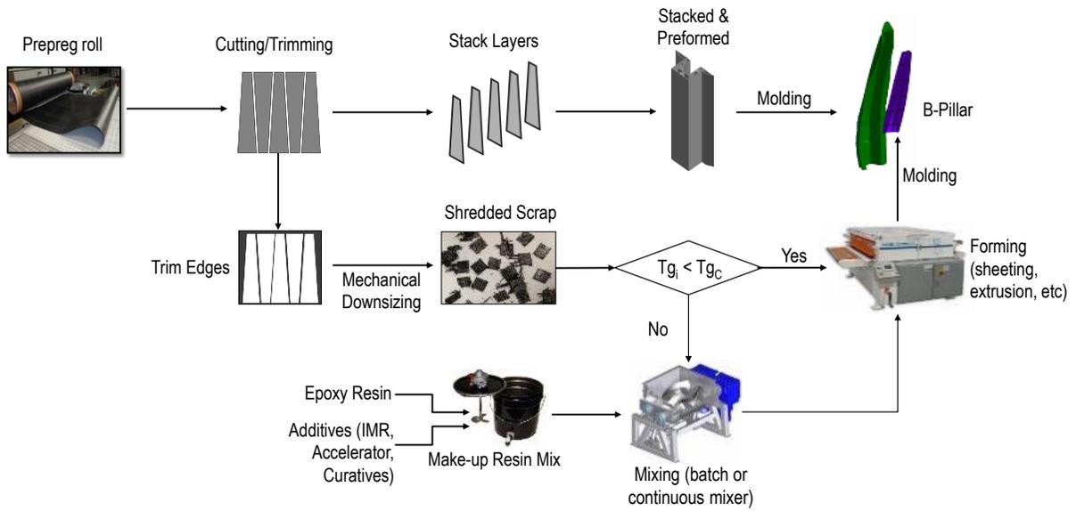
Figure 2: Process schematic of the proposed scrap reutilization method
