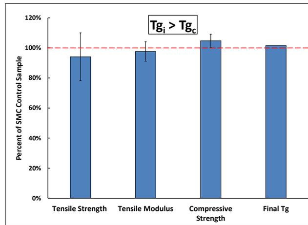
Figure 4: Relative properties comparison between material made from DLF process and molding compound prepared from the trim scrap when the trim scrap  $Tg_i > Tg_c$
