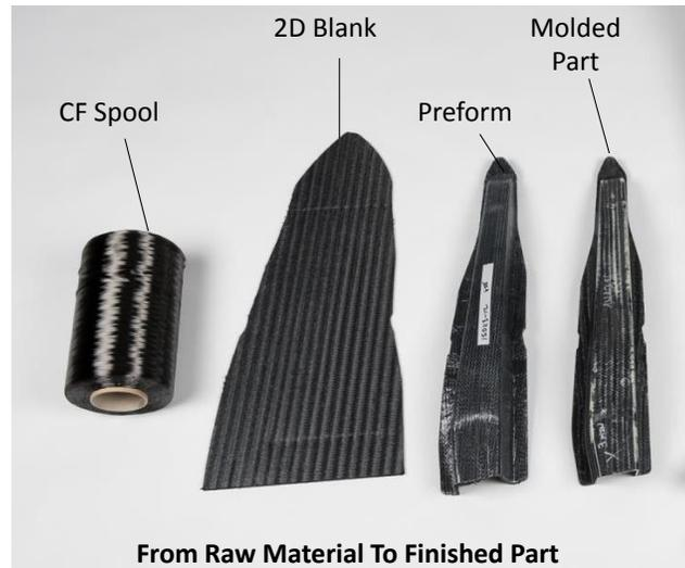
Figure 1: B-Pillar Insert (Raw material to finished part)
