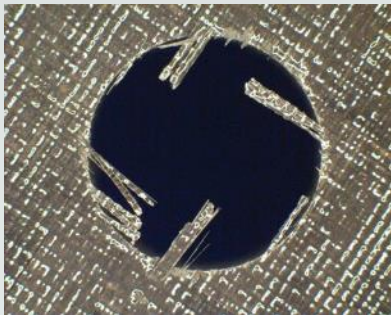
Delamination in composites due to hole-drilling, Gardiner, Composites World , (2012)
