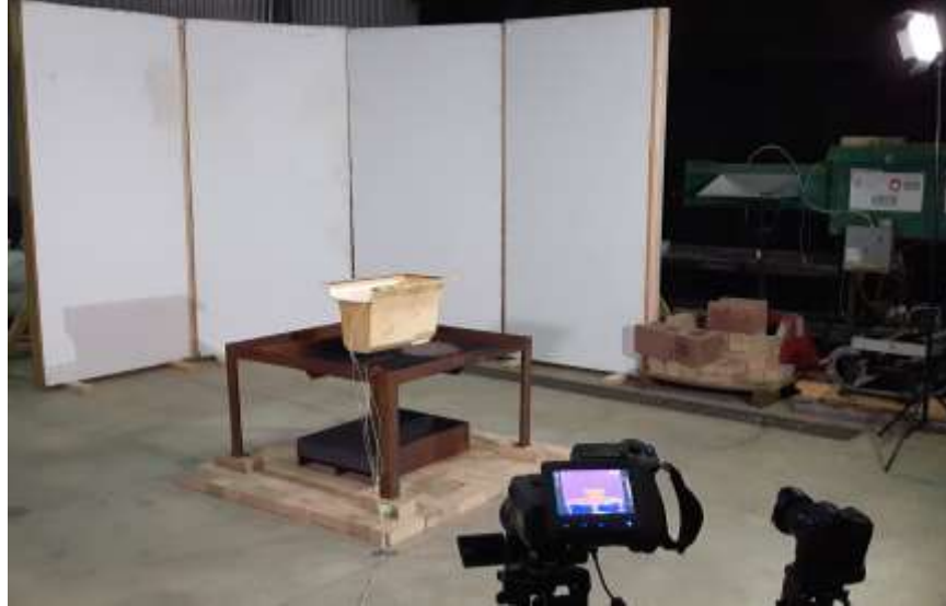
Figure 1 – Fire testing setup after ECE R100 & GB/T 31467.3
