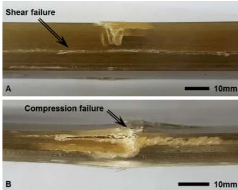
Figure 3 – Undesirable failure modes with different beam thicknesses a) 22mm b) 11mm
