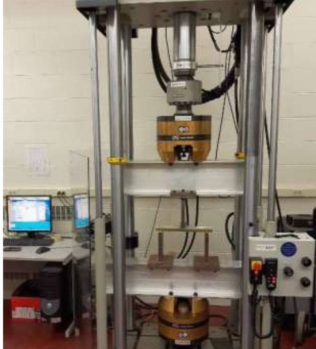
Figure 1 – Fatigue testing setup for thick component testing
