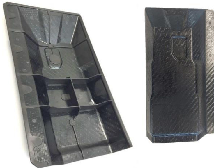
Figure 1: Test geometry for organic sheet components allowing in line-measuring of the thermoplastic composite's temperature during overmolding.
