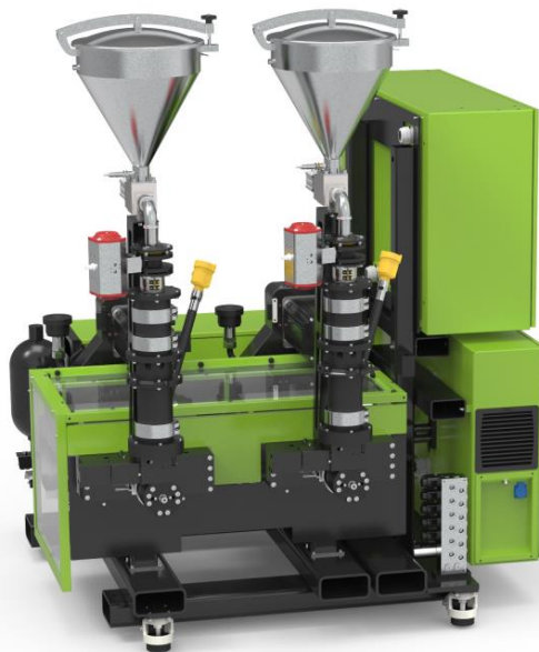
Figure 4: Reactive dosing unit used for the processing of epsilon-caprolactam within the scope of the T-RTM technology. The in-situ polymerization is leading to thermoplastic composite components with polyamide-6 matrix.
