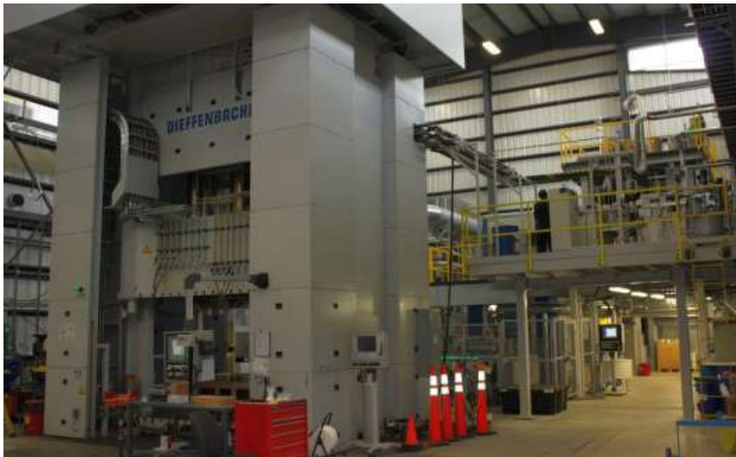
Figure 2: FPC equipment- press and HP-RTM
