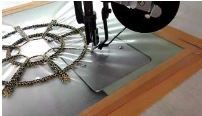
Figure 10: Tailored-fiber placement of commingled yarn.
