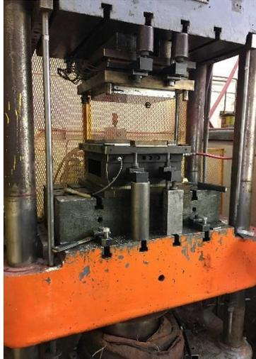
*Figure 2: Hot press and mold for plaque manufacturing*
