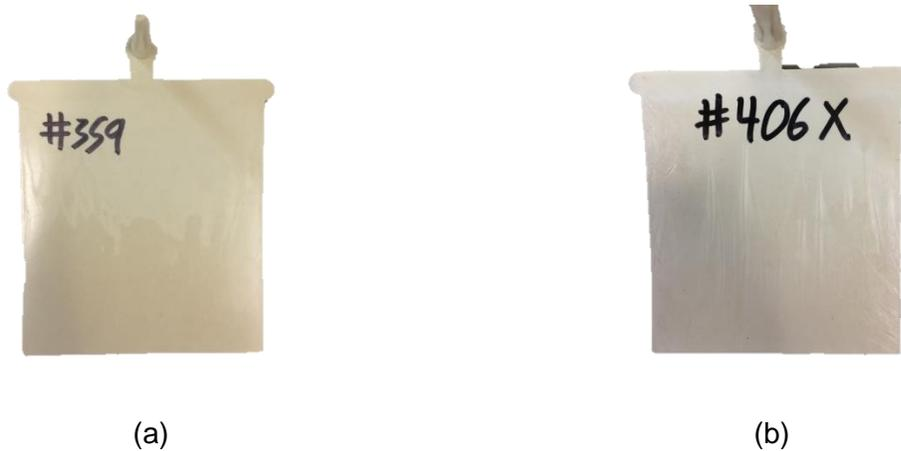
Figure 5: Injection molded end-gated plaques, molded using (a) 56.0 wt.% HX3000/PP and (b) 50.0 wt.% HX3000/HX8000 TPIC pelletized strands.
