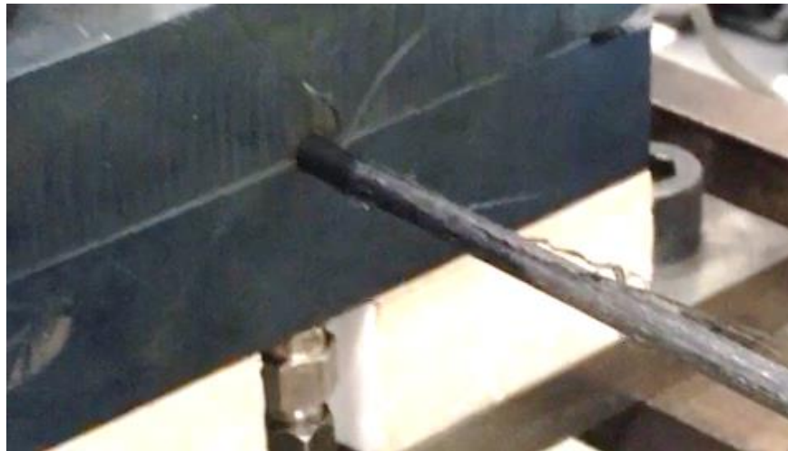
Figure 6 Image of the cooling die's exit during PEI-300 experiment. The image is showing dry carbon fibers detaching from the pultruded beam as it leaves the cooling die.
