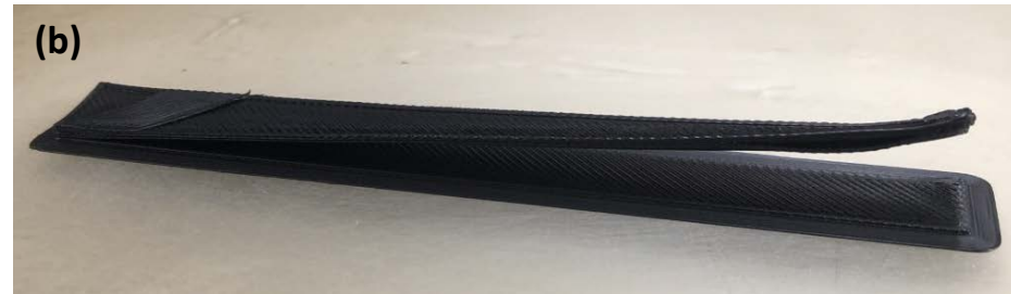
Challenges faced during before optimization of printing parameters: (a) warpage and (b) delamination
