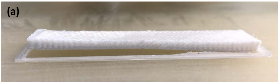
Challenges faced during before optimization of printing parameters: (a) warpage and (b) delamination
