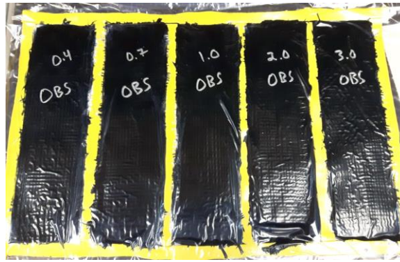
Figure 2: A set of color pigment concentration samples prior to being cured; each sample is 300 x 80 x 2.5 mm
