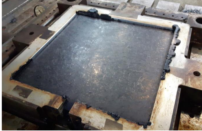
Figure 5: Sample phenolic/glass SMC plate molded at the Fraunhofer Project Center, dimensions 457x457x2.5 mm
