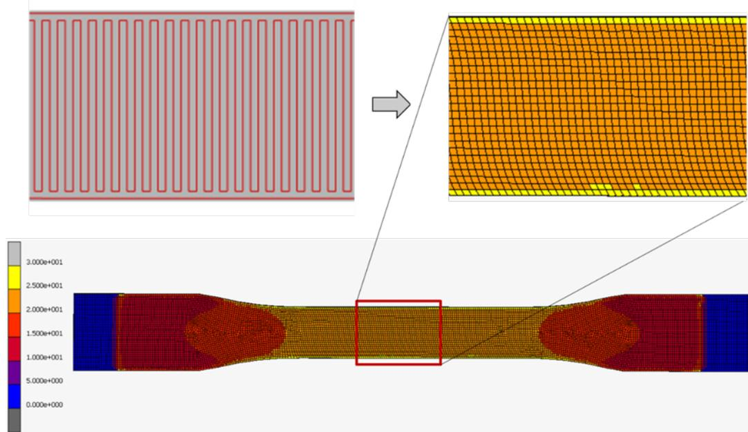
Figure 3: Von Mises stress [MPa] of the dumbbell tensile test
