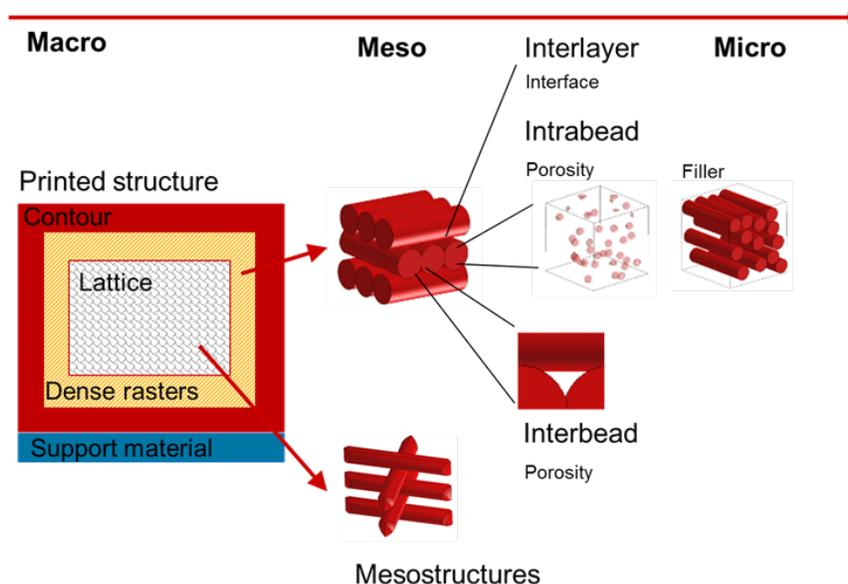
Figure 1: Additive manufacturing is a multiscale challenge (illustrated for the FFD process)
