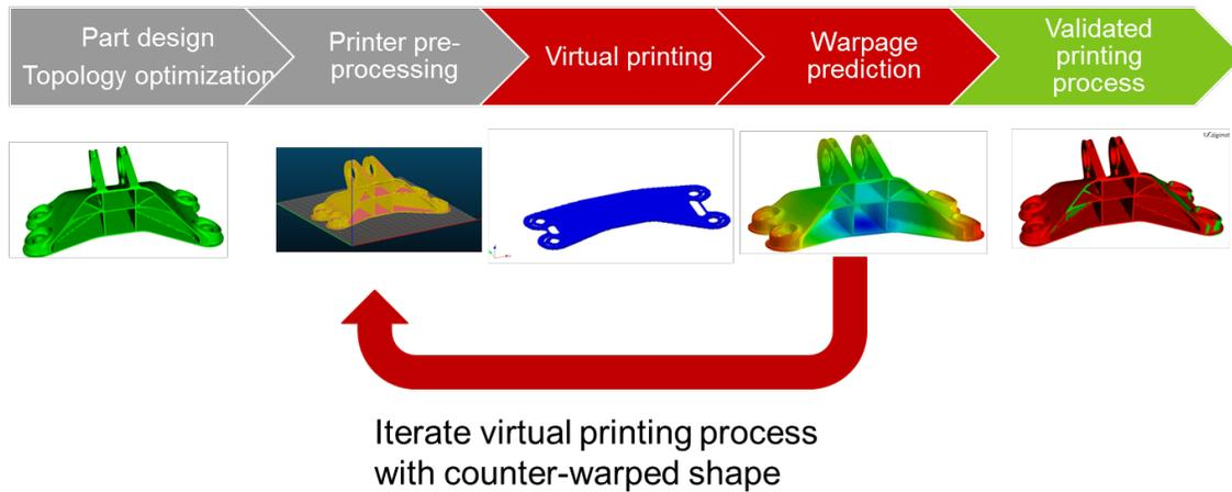
*Figure 2: Complete workflow for optimal printing*
