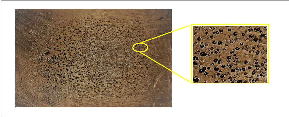
Figure 2: Cross-section of the cross-tie with varying density and cell sizes
