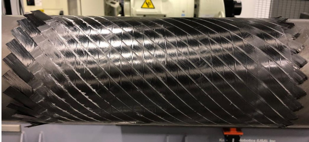
Figure 4- Part made with silicone compaction roller showing 45° ply during fabrication
