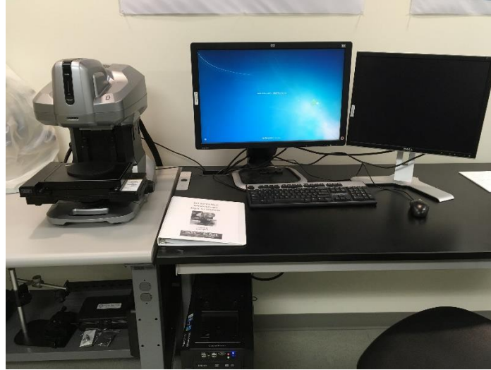
Figure 7. Keyence VR-3000 One-shot 3D Measurement Macroscope .
