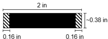
Figure 4. Dimensions of the 3D printed sample to be burned off.
