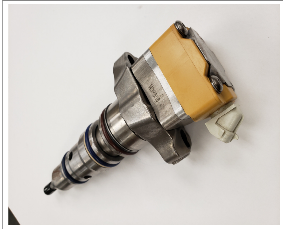
Image 1. Fuel injector with EMC (yellow) encapsulated solenoid.
