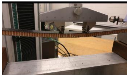
Figure 7. Sandwich beam under 4 Point Bending Setup
