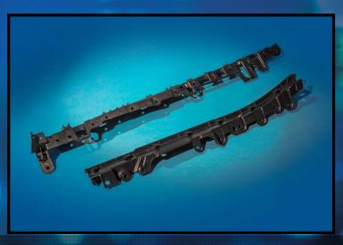
This is the first thin wall (2.0mm nominal wall construction) structural appearance application that resulted in lower cost, lighter weight, improved appearance and better performance. Injection molding with sequential valve gating and 20% long glass fiber PP enabled this application. A 20% mass savings and a 8% cost savings resulted.
