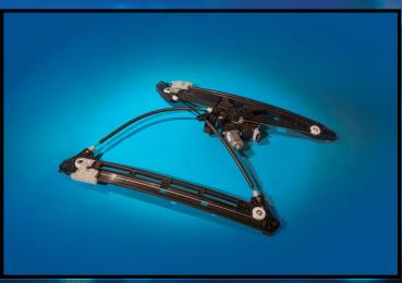
This is the first significantly lower-weight window regulator without compromise to safety, assembly time, strength or cost. By utilizing thermoplastics, the weight is similar to regulators that use aluminum guide rails but no more expensive than conventional regulators that use steel guide rails. The weight was decreased by 23% on the front doors and by 14% on the rear doors.
